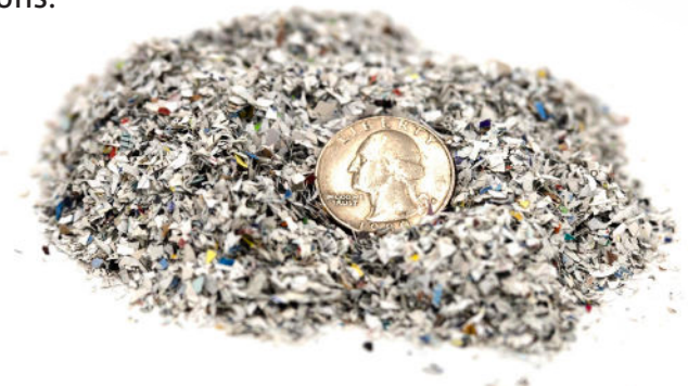
Paper disintegrated to NSA mandated particle using a 3/32" screen for classified and CUI data
