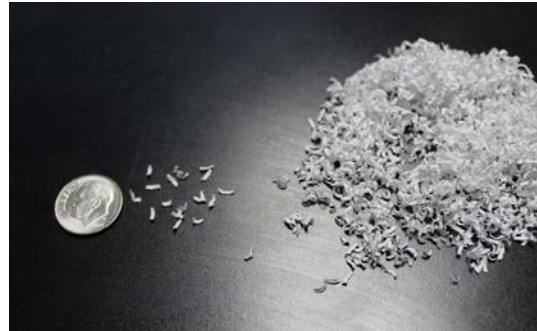
The NSA mandates that classified paper be destroyed to a particle size of 1mm x 5mm or less (DIN P-7)
