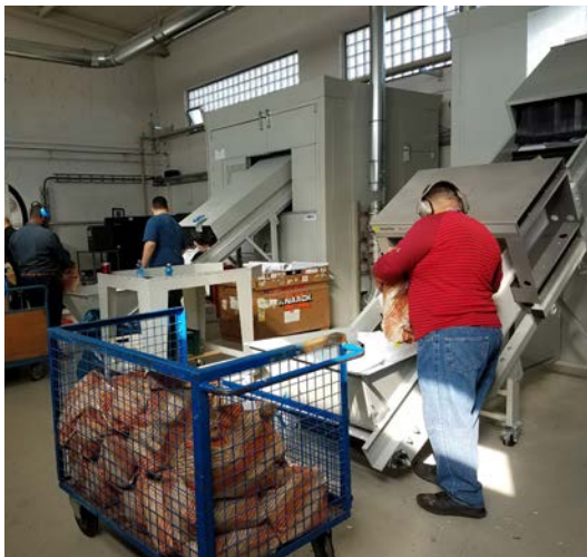
Centralized military high security destruction facility utilizes two disintegrators with briquetters
