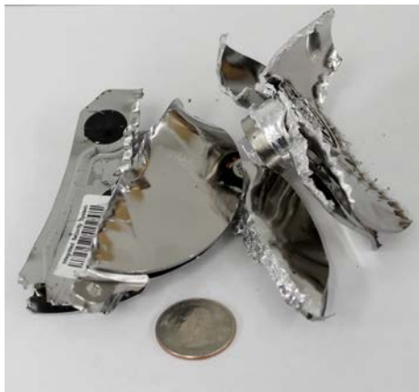
Standard final particle size for an HDD shredder is 1.5", while 1.0" and 0.75" options are also available
