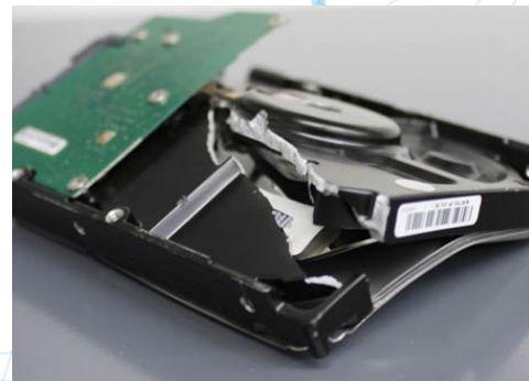
HDDs that have been both degaussed and crushed are unrecoverable
