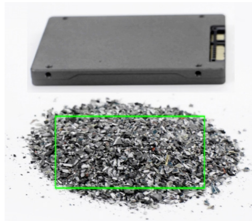
Per the NSA, classified SSDs must be destroyed to a particle size of less than 2mm
