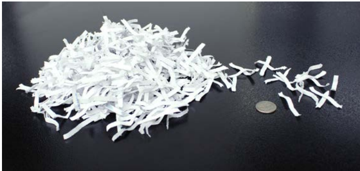
DIN level P-4 particle (4mm x 40mm) is acceptable for sensitive and confidential non-classified paper
