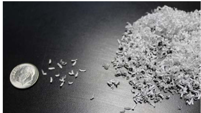
DIN level P-7 particle (1mm x 5mm) is the requirement for all classified and CUI paper
