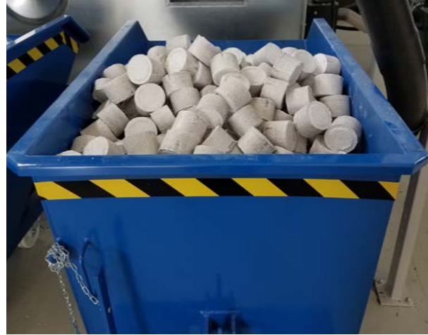
Briquetting reduces waste by over 90% and allows the shredded material to be recycled
