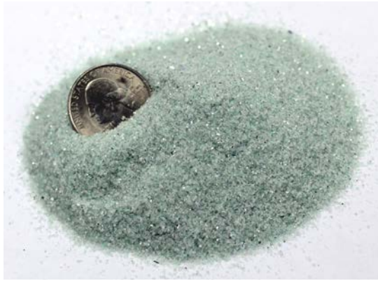
The 2018 NSA EPL mandates that classified DVDs and BDs be destroyed to a particle size of less than 2mm
