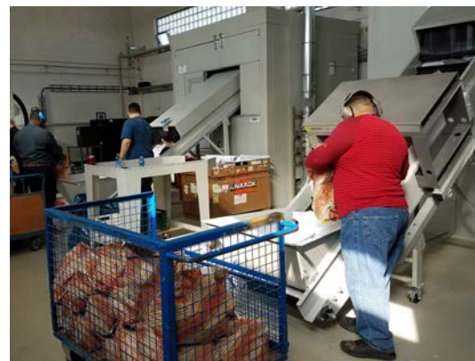
Centralized military high security green destruction facility utilizes two disintegrators with briquetters
