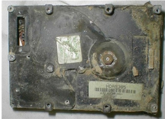
The hard drive recovered from the Space Shuttle Columbia
