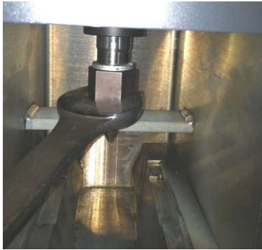
Turn anvil with 1-1/2" open-end wrench
