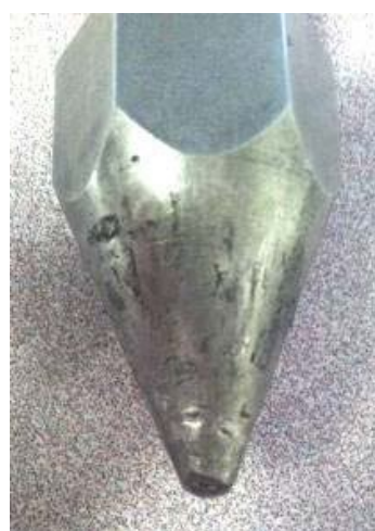
Worn HDD Anvil
