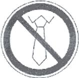
3. Do not operate or come in close proximity to this equipment wearing long hair, necktie, loose clothing or jewelry, which may activate a photoelectric on/off switch and/or be pulled into the machine!
