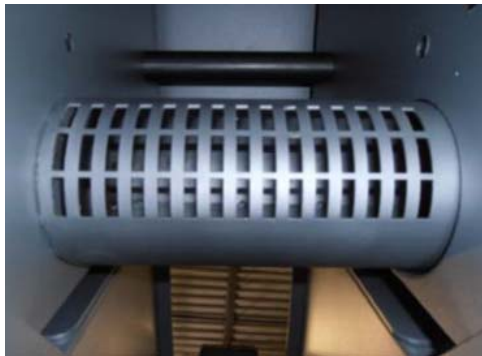
Bottom of Air Inlet
