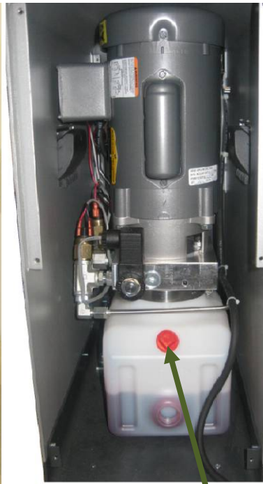
Remove Reservoir plug and replace with the supplied Breather plug, can be located in bag in crushing chamber
